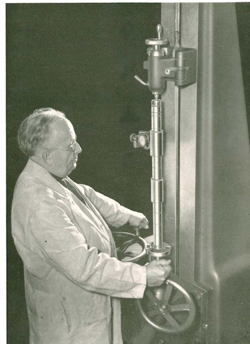
Testing the assembled arbor for concentricity. The testing machine was especially designed for this operation.
