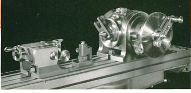
UNIVERSAL DIVIDING HEAD . . . for milling accurately spaced slots, drilling holes, milling master cams, or any type of job which requires close accuracy on the arc of a circle.
