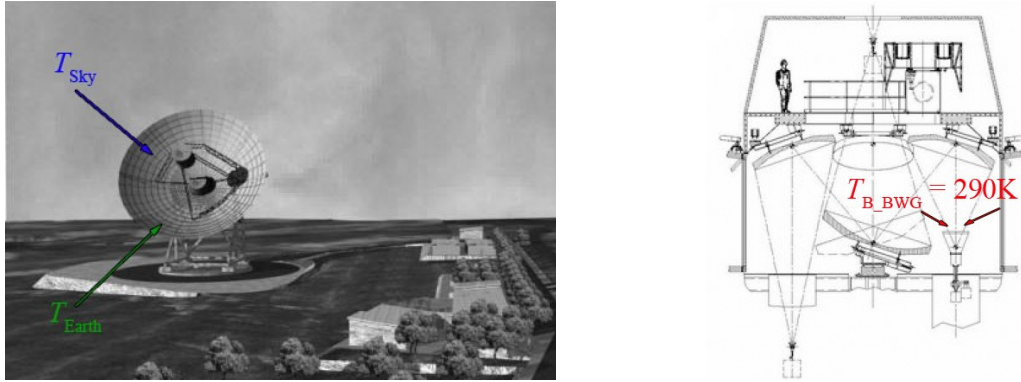
Fig. 3: Contributions to the SRT antenna temperature: sky and earth (left) and beam waveguide room (right).
