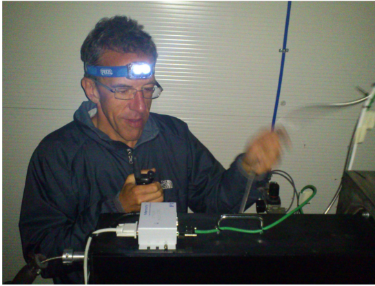
Figure 3.3 Human-driven fiber-shaker, used to decrease the fiber modal-noise during the observations.
