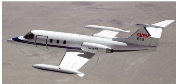
Aircraft in Stratosphere NASA Learjet, 30cm telescope, 1968- IR absorption and emission features
